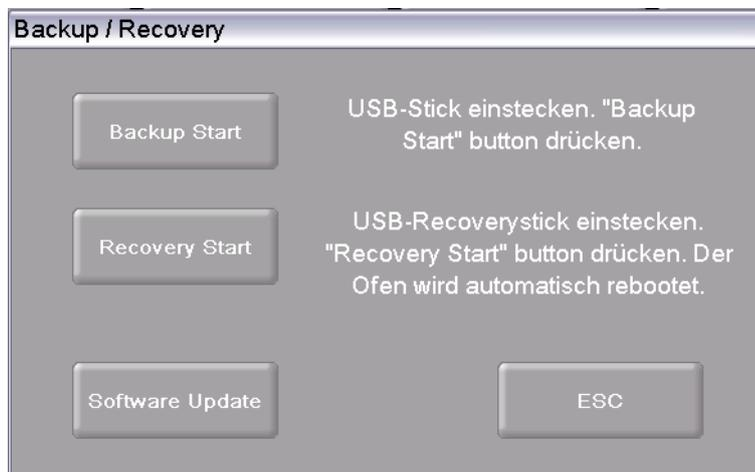
Fig. 5-42 Setup > Backup / Recovery
