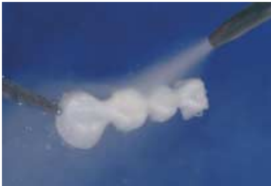
Before veneering, clean framework under running water or with the steam jet and dry. The framework must not be blasted with Al 2 O 3 .
