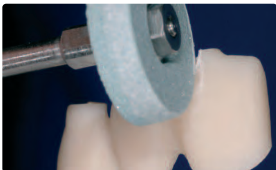
Smooth out the attachment points of the sprue using low speed and light pressure
