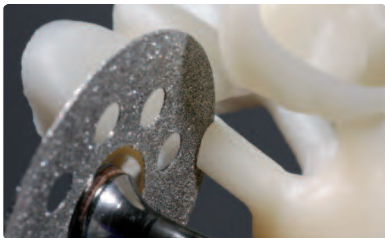
Wet the area to be ground and use a fine diamond disk to cut the sprues
