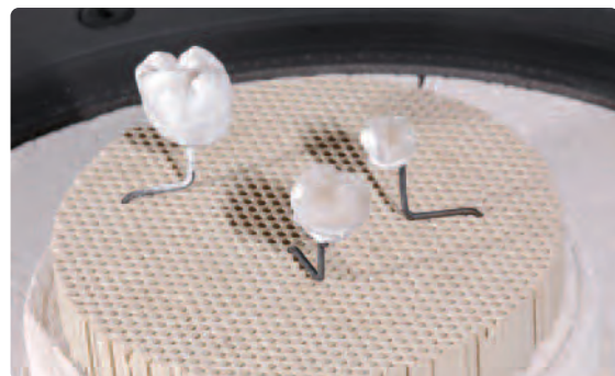
Conduct the Glaze firing on a honey-combed tray with the corresponding parameters
