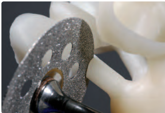
Wet the area to be ground and use a fine diamond disk to cut the sprues
