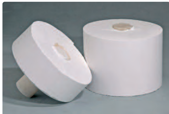
Separate the investment ring using a separating disk and break at the predetermined breaking point
