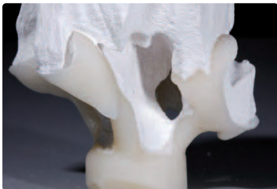
Fine divestment is carried out with polishing beads at 2 bar (30 psi) pressure
