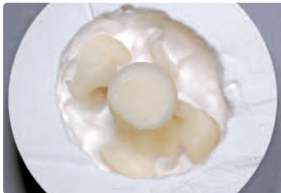
Rough divesting with polishing jet medium at 4 bar (60 psi) pressure until the objects become visible
