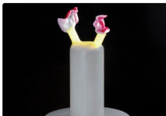
On the IPS investment ring base, attach sprues in the direction of flow of the ceramic and to the thickest part of the restorations
