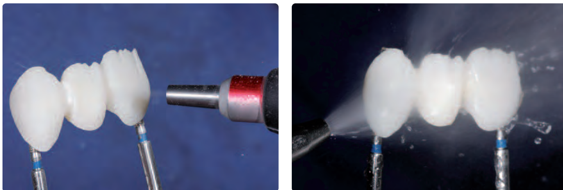
Blast the restoration with Type 100 Al 2 O 3 at 1 bar (15 psi) pressure. Thoroughly clean the surface with a steam jet prior to the wash firing and subsequently dry.
