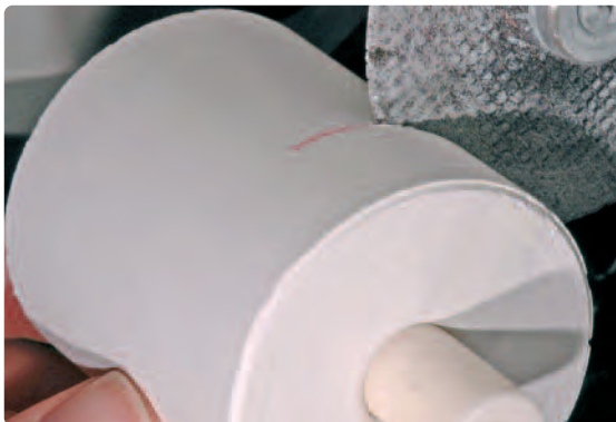
Separate the investment ring using a separating disk and break at the predetermined breaking point
