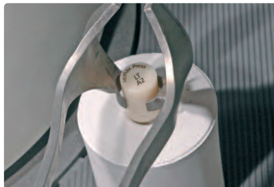
Place the cold IPS e.max Press ingot into the hot investment ring, with shade imprint facing upward
