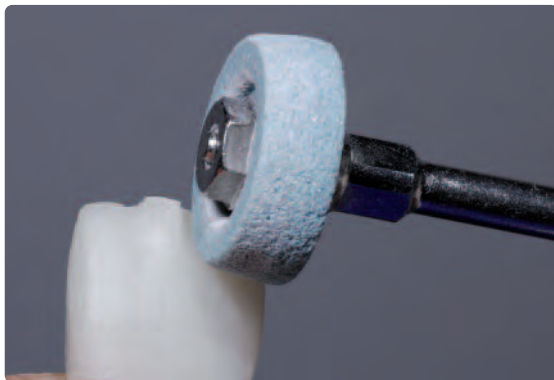
Smooth out the attachment points of the sprue using low speed and light pressure
