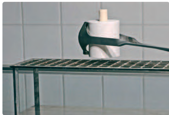
Once the press program is completed, place the hot investment ring on the cooling grid using the investment ring tongs and allow it to cool to room temperature
