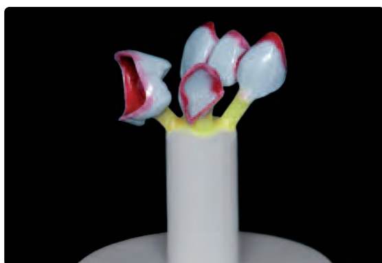
On the IPS investment ring base, attach sprues in the direction of flow of the ceramic and to the thickest part of the restorations
