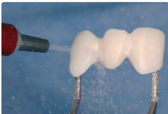
Blast the restoration with Type 100 \text{Al}_2\text{O}_3 at 1 bar (15 psi) pressure. Thoroughly clean the surface with a steam jet prior to the wash firing and subsequently dry.
