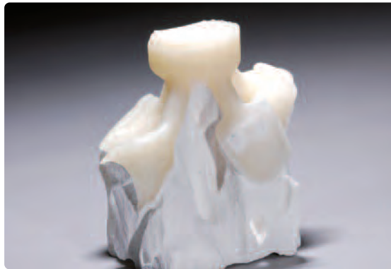
Fine divestment is carried out with polishing beads at 2 bar (30 psi) pressure
